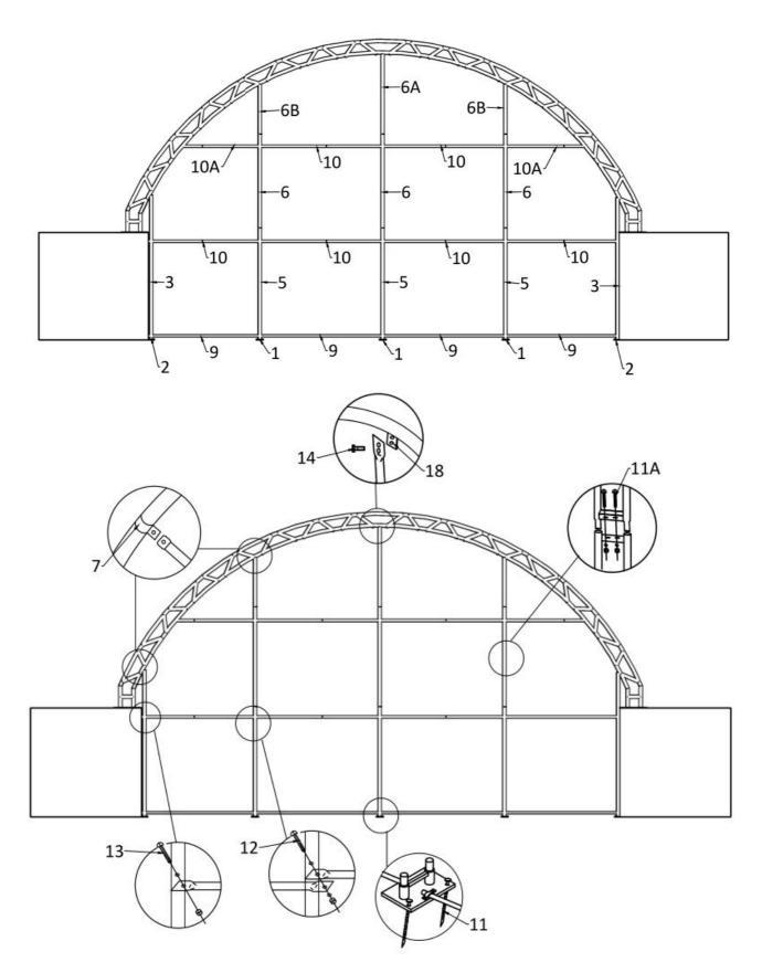
According to above Figure to find out all spare parts for back wall, connect them together by use screw, make sure the spacing. There are stake pegs for base plates.
