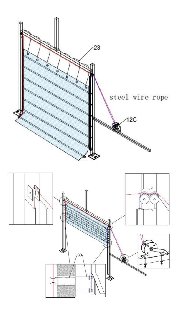
After assembly the front wall, find out the front cover, use ropes to tie the front cover to the front wall. There are some dropping tubes (No.33) need to be insert into the door cover, use steel wire to insert into all these dropping tubes one by one, and go through the pully from top to bottom & from bottom to top. Tie the end of the steel wire to the winch wheel. Thus when you move the winch wheel, the door could be go up and down.
