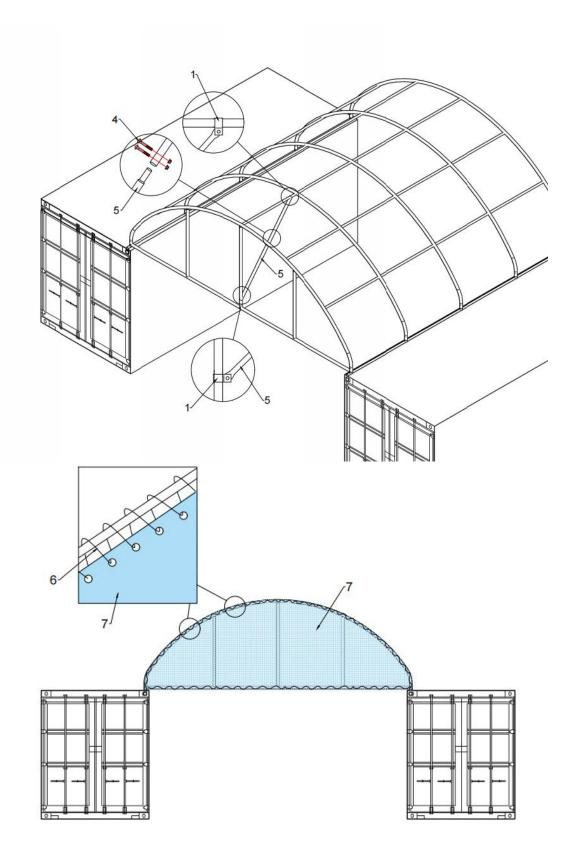
Assembly the frame first according to above drawing. Then use ropes No.6 to tie the cover to the frame.
